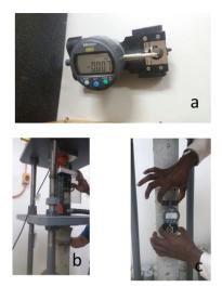
Figure 3: (a) Demec strain gauge (b) Hydraulic jack, load cell positioned to induce predetermine load intensity on concrete sample (c) Creep strain reading using the Demec gauge
