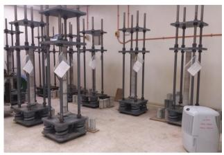
Figure 2: Compressive creep rig with specimen under sustained load
