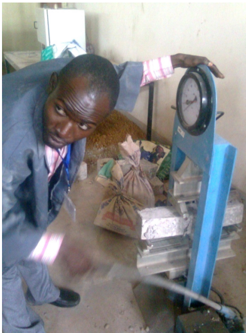
Plate 1: simple concrete beam tested
