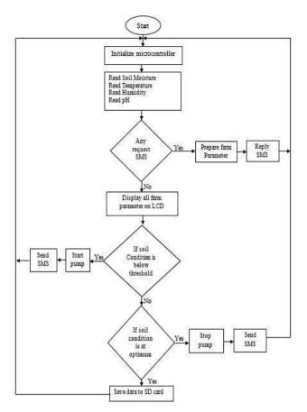
Figure 2: Flowchart of the control system
