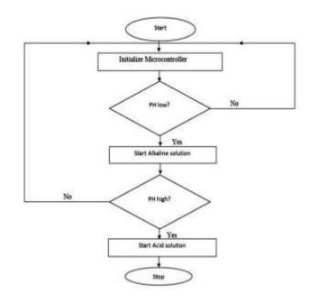
Figure 7: Flowchart of the pH sensing
