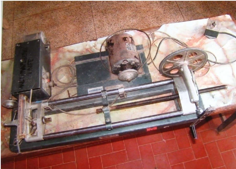
Plate VI: Hounsfield Tensometer (Monsanto Tensometer, type W, Serial No 10055)
