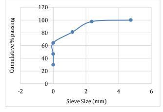
Fig. 3. PSD of QDP (as supplied).
