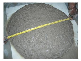
Fig. 1. Slump flow test measurement.
