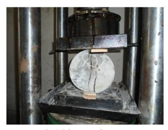
Fig. 7. Splitting tensile testing.
