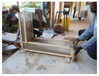
(b) L-box flow test
