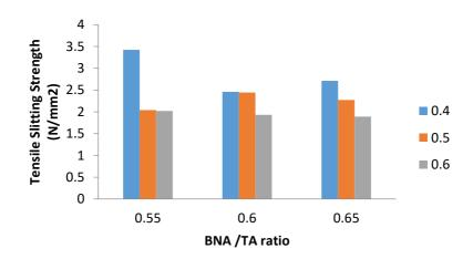
Figure 4: Splitting tensile Strength results for all mixes
