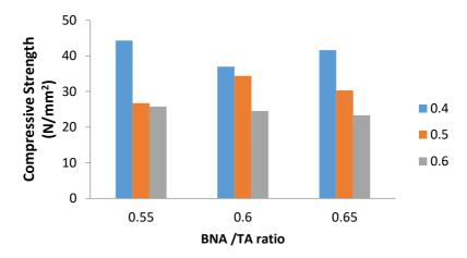
Figure 2: Compressive Strength results for all mixes
