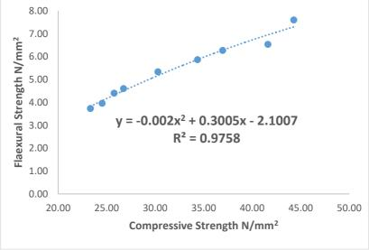
Figure 5: Relationship between compressive and flexural strength.
