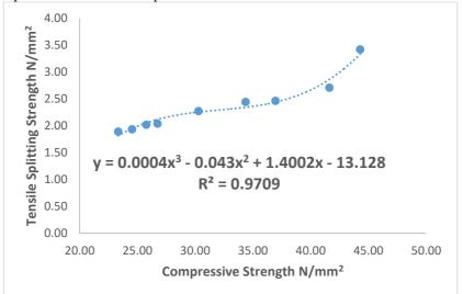
Figure 6: Relationship between compressive and splitting tensile strength.
