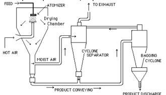
Figure 4. Spray drying process.
