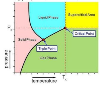
Figure 3. Supercritical fluid diagram.
