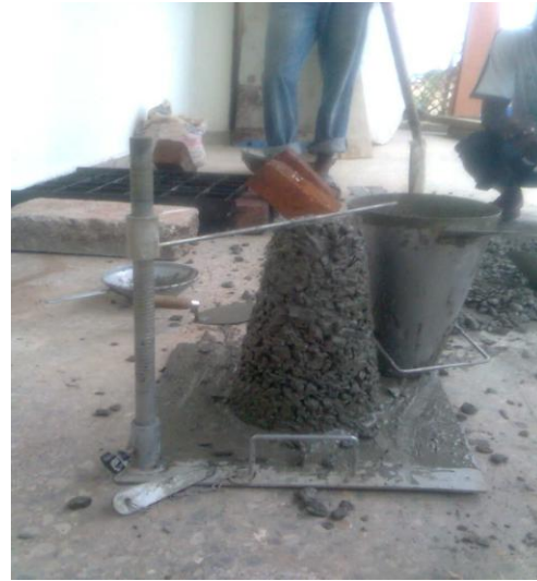
Plate 4: Slump for CPA/OPC Laterized concrete
