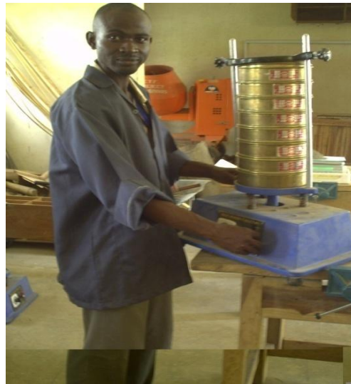
Plate 6: sieve shaking of aggregates
