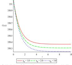
Fig 8: Variation of Contaminant concentration with Time for Different Values of Initial Velocity
