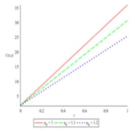
Fig 9: Variation of Contaminant concentration with Space for Different Values of Initial Velocity
