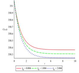
Fig 4: Variation of Contaminant concentration with Distance *x* for Different Values of Decay Parameter
