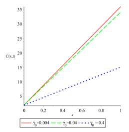
Fig 3: Variation of Contaminant concentration with Time for Different Values of Decay Parameter
