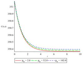
Fig 5: Variation of Contaminant concentration with time for Different Values of Zero Order Source Coefficient
