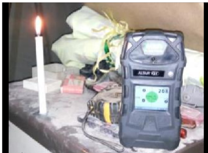
Plate I: Measuring CO Emission from Candle Source: Authors 'field work, 2018.
