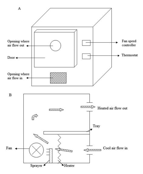
FIG. 1. STRUCTURE OF CABINET DRYER (A) EXTERNAL STRUCTURE (B) INTERNAL STRUCTURE
