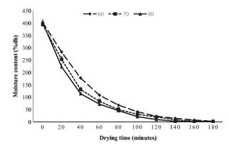
FIG. 4. DRYING CURVES OF FOAMED CORN SLURRY AT DIFFERENT DRYING TEMPERATURES AND DRYING TIME Note: Vertical lines show standard deviation from the mean.
