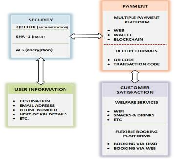
Figure 2: Block Diagram of Secure Bus Service System
