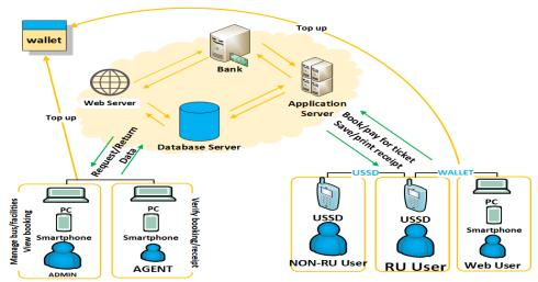
Figure 1: Architecture of Secure Bus Service System
