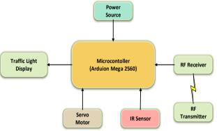
Figure 3: Block diagram for density-based traffic control system
