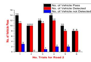
Figure 10: Performance measurement for Road 2 with IR Sensor
