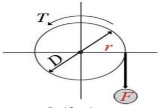
Figure 4: Torque of servomotor
