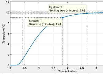
Figure 4 Temperature response of CRAC to unit step input (without compensator)
