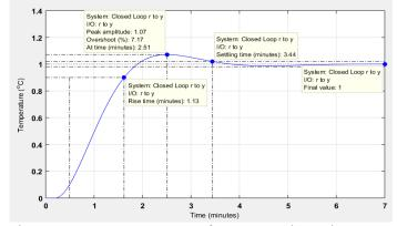
Figure 5 Temperature response of CRAC to unit step input (compensator)
