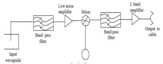
Fig. 1.0: Low noise block down converter diagram
