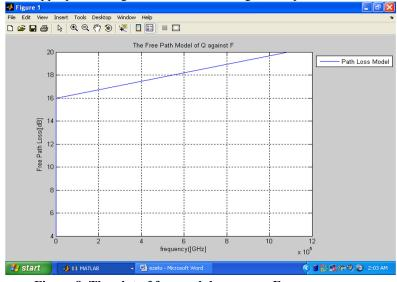
Figure 8 The plot of free path loss versus Frequency
