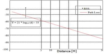
Figure 3: Sample path loss measured by IEEE 802.11 pc Card
