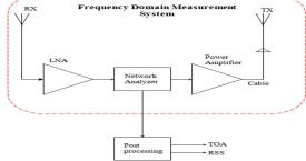
Figure 5: Frequency domain measurement system
