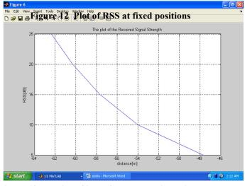
Figure 13 Received Signal Strength against Distance
