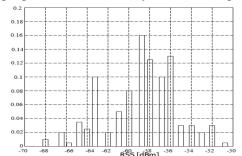
Figure 4: RSS distribution at a fixed location obtained by a WiFi measurement system.
