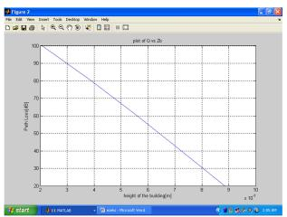
Figure 9 The plot of Path loss against Building height
