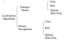
Figure 6: Classification of localization algorithms.
