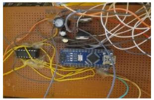
Figure 11. Robot connection on vero board
