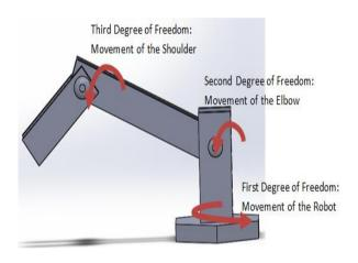
Figure 10. Robot arm degree of freedom
