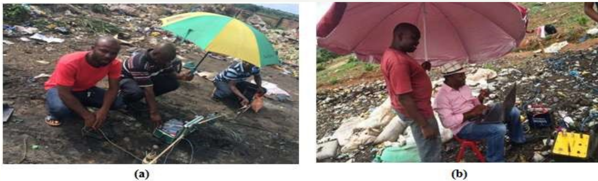
Figure 4: Data acquisition within the study area: (a) VES layout; (b) Seismic Refraction Tomography layout
