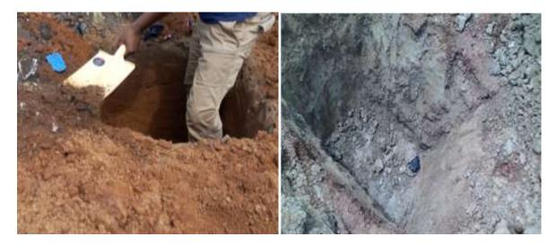
Plate II: Digging of the Trial Pits and a Trial Pit within the Study Area
