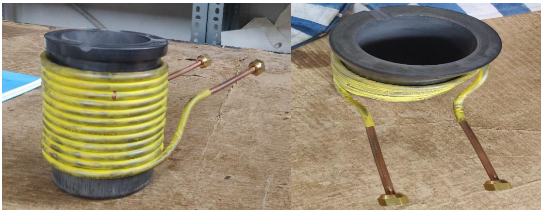
PLATE III: Heating Coil for Induction Furnace and Crucible
