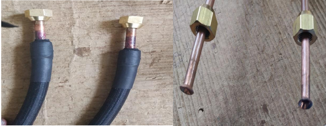
PLATE IV: Flexible Heating Coil Hose and Shift Heating Coil Input and Output
