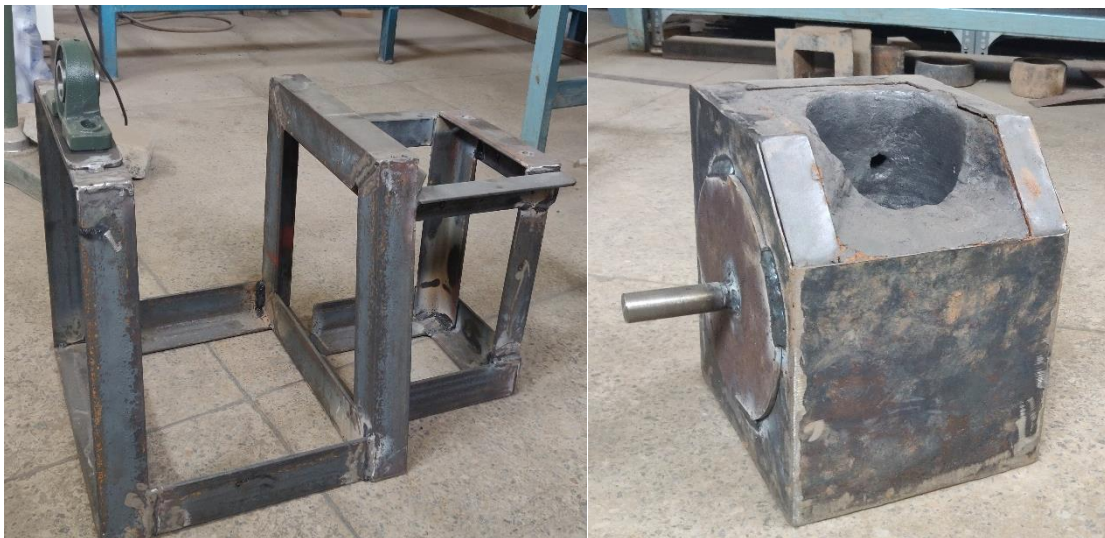
PLATE I: Frame and Crucible Housing for Induction Furnace
