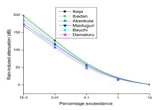
Figure 8: Rain-induced attenuation at 40 GHz uplink, circular polarisation
