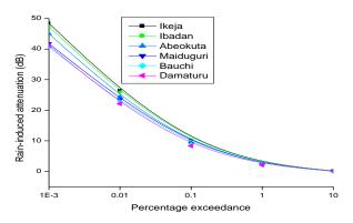
Figure 2: Rain-induced attenuation at 14 GHz uplink, horizontal polarisation
