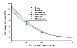
Figure 9: Rain-induced attenuation at 11 GHz downlink, vertical polarisation
