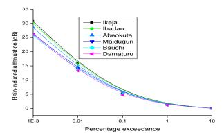
Figure 1: Rain-induced attenuation at 11 GHz downlink, horizontal polarisation
