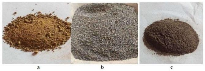
**Figure 3.1:** (a) Clay soil; (b) Unpulverized volcanic ash; (c) Pulverized volcanic ash XRay fluorescence (XRF) tests were also carried out on the clay soil. The tests were conducted in Ithemba Laboratory, Somerset West, South Africa and Electron Microscope Unit, University of Western Cape, Cape Town, South Africa. Phase characterization of the minerals and estimate of the average crystallite size of the various synthesized materials were conducted on a Bruker AXS D8 XRD system.
