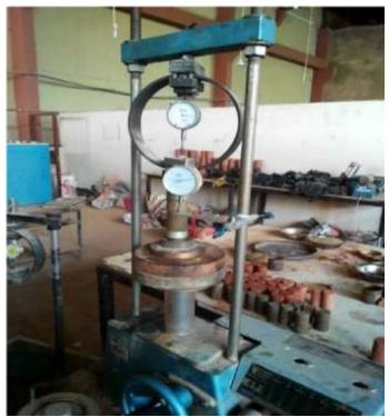
PlateI: Unconfined compressive strength test
