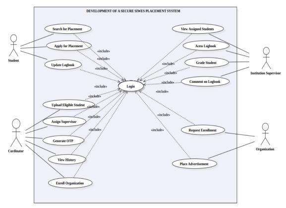
Fig.2. Use Case Diagram of the system. Source: (Author)
