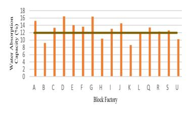
Water Absorption Capacity of Blocks
