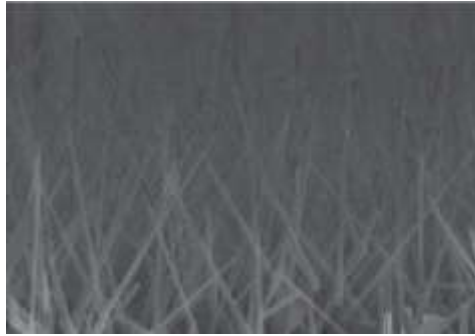
Figure 2.2: Scanning electron microscope (SEM) image of nanostructured ZnO nanowires
