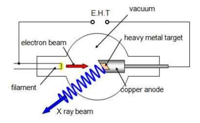
Figure 2.1 Schematic of an X-ray tube (Hrishikesan, 2018).
