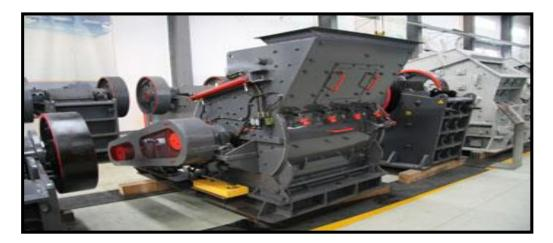
Plate VII: Hammer Crusher Source: Shanghai Joyal Machinery Co Ltd (2019)
