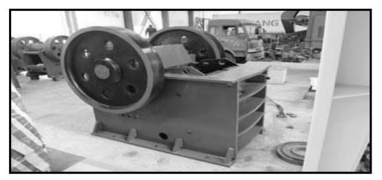
Plate II: PE Jaw Crusher Source: Shanghai Joyal Machinery Co Ltd (2019)
