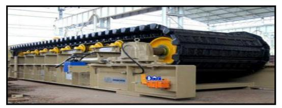
Plate V: BWZ Series Heavy Duty Apron Feeders Source: Shanghai Joyal Machinery Co Ltd (2019)
