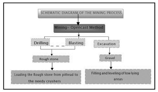
Figure 2.1: Method of Open-Cast Quarry Mining Source: (Annadurai *et al.*, 2010)
