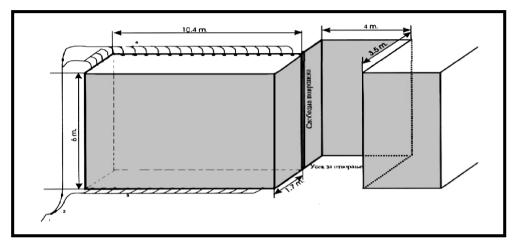
Figure 2.2: Method of Horizontal and Vertical Drianed Holes in Quarry Source: (Dambov *et al.*, 2013).
