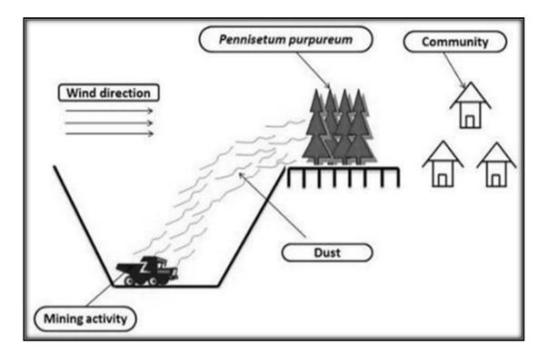
Figure 2.4: Dust Barrier Model Source: Mbandi (2017)
