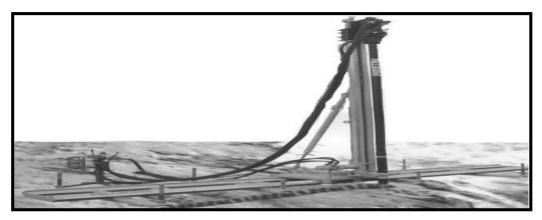
Plate I: Drilling machine TBC SLOT Source: (Dambov *et al.*, 2013).
