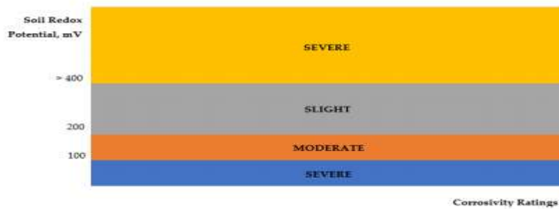
Figure 2.14: The Relationship between Soil Corrosivity and the Redox Potential (Arriba-Rodriguez et al. , 2018)
