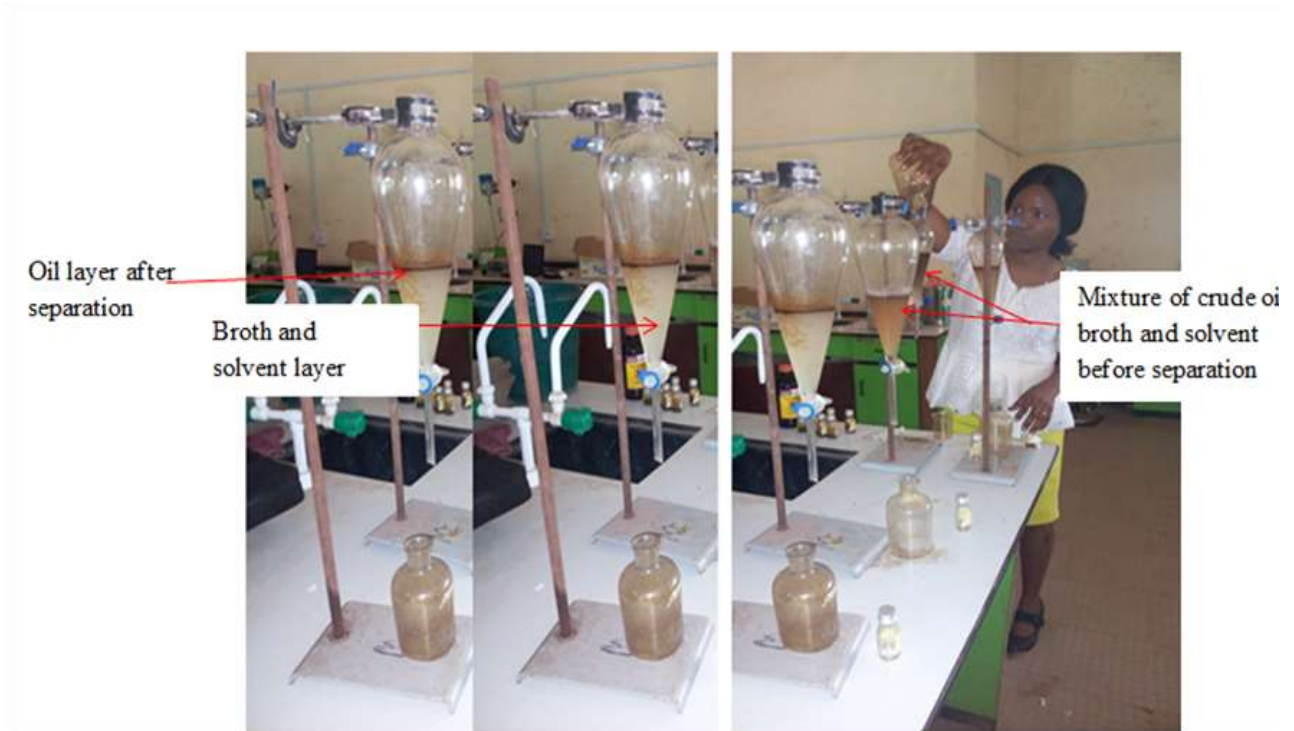
G1: Extraction of residual crude oil after microbial degradation in a liquid medium (broth
