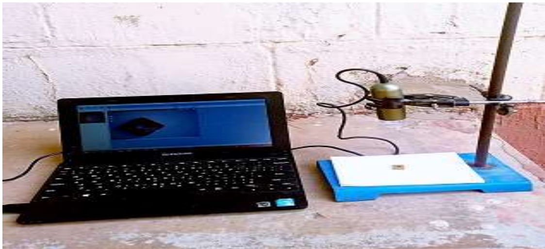
Figure 3.3: Set up component of digital microscope tool wear measuring device
