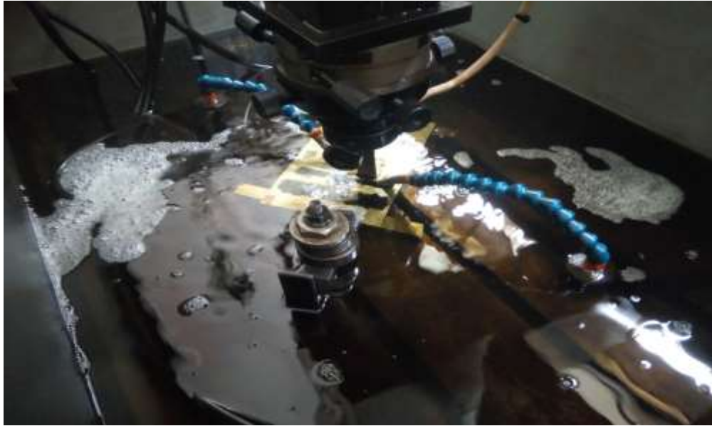
Plate XII: Cutting with Wired EDM
