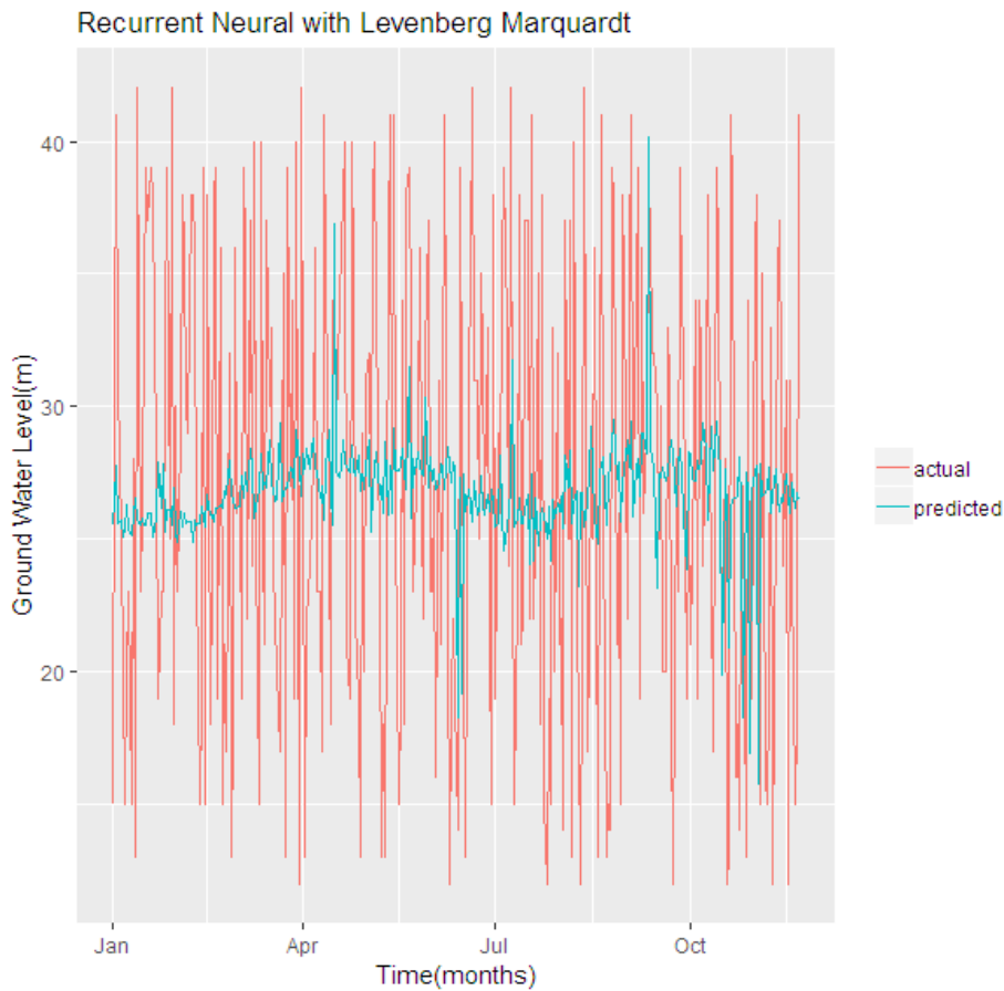
Figure 4.13: Hydrograph of the groundwater for the third best performance algorithm in Bida
