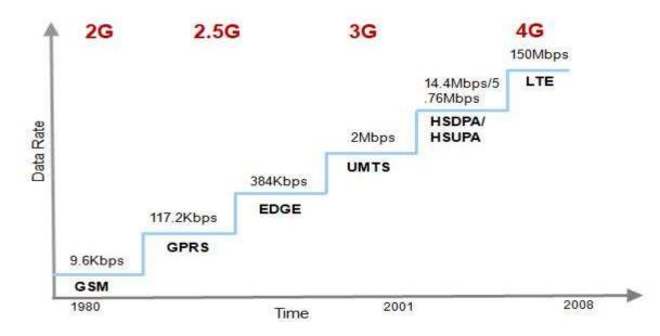
Figure 1.2 Evolution of Mobile Network Technology. Source: (Qing, 2017)
