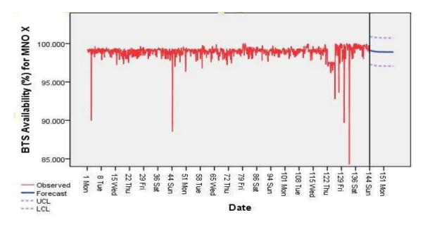
Figure 4.12 Predicted BTS Availability for MNO X Using ARIMA (1,0,1) Model. Similarly, the predicted BTS availability are presented in figures 4.12 and 4.13 using ARIMA (2,0,4) and ARIMA (0,1,1) respectively.
