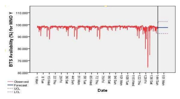
Figure 4.13 Predicted BTS Availability for MNO Y Using ARIMA (2,0,4) Model
