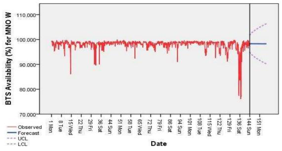
Figure 4.11 Predicted BTS Availability for MNO W Using ARIMA (0,1,3) Model.
