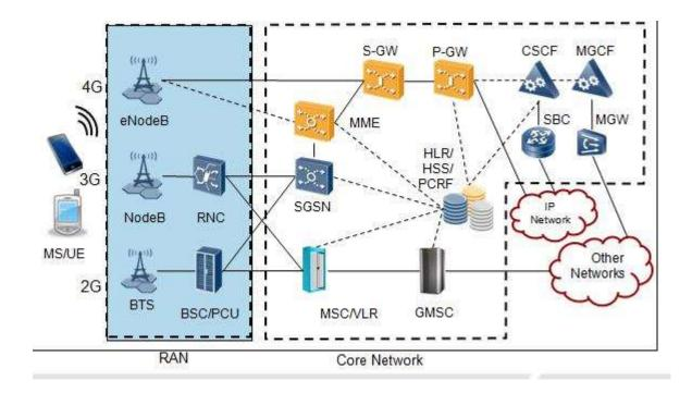
Figure 1.1 A Typical Telecommunication Network. Source: (Qing, 2017)
