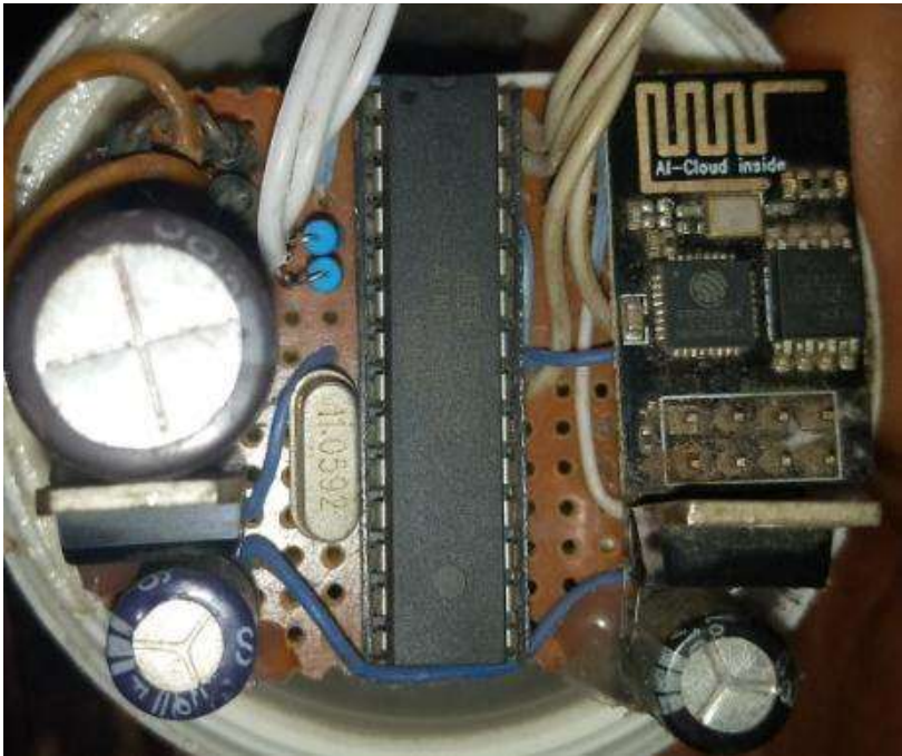
Plate XIV: Complete IoT Device for Human Monitoring
