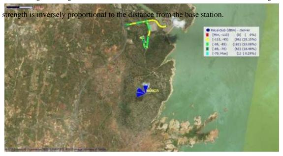
Figure 4.1: Received signal strength for Network A
