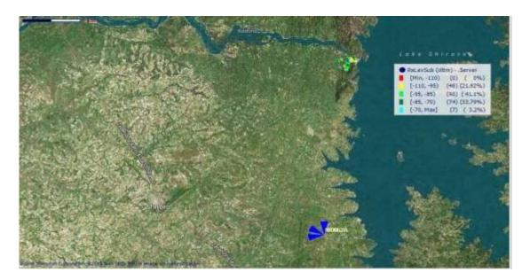
Figure 4.7: The received signal strength for network D
