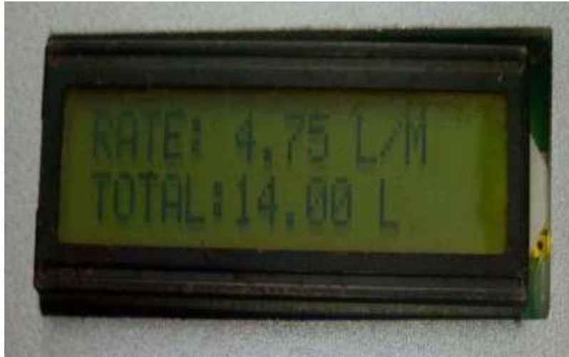
Plate IV: Display of Developed IoT Water Meter
