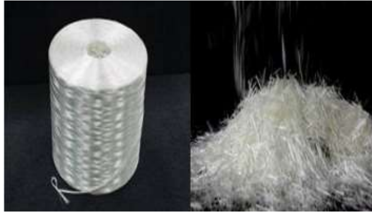
Plate IV: Typical AR-glass fibres used in concrete
