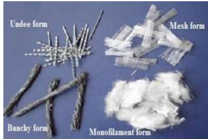
Plate V: Typical forms of synthetic fibres used in concrete
