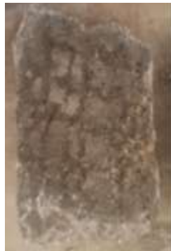
(a) The old concrete prism sample halved at 30° (halved 100 x 100 x 200 mm) Grooved surface exposes aggregate
