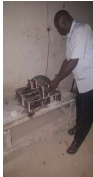
(c) Vibrating halved (100x 100 x 200 mm) prism in form
