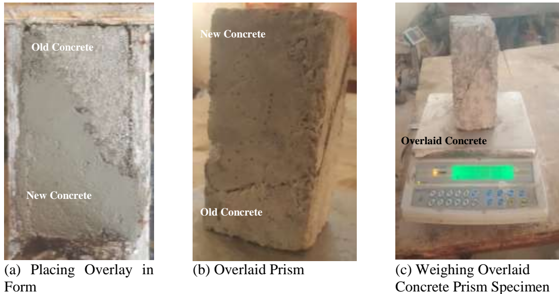
Plate XV: Overlaid Concrete Prism Specimen for Interfacial Bond testing
