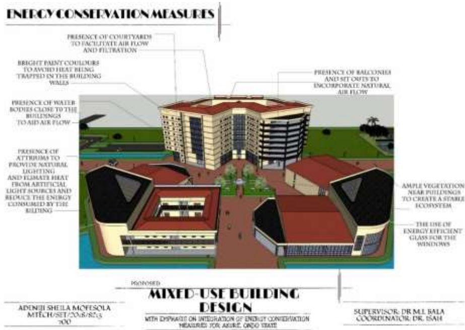
Plate XXVII: Energy conservation measures for cooling Source: Author's work (2020)
