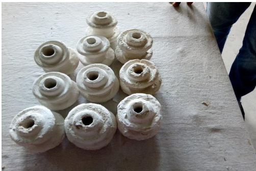
(a) Casted specimen; unfired, unglazed and unfelted.
