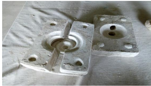
Fig. 2: Casting mould made of POP
