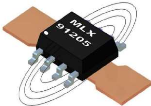
Figure 3.8: MLX91205 Medium Current Sensing Configuration ( MELEXIS MLX91205, datasheet )
