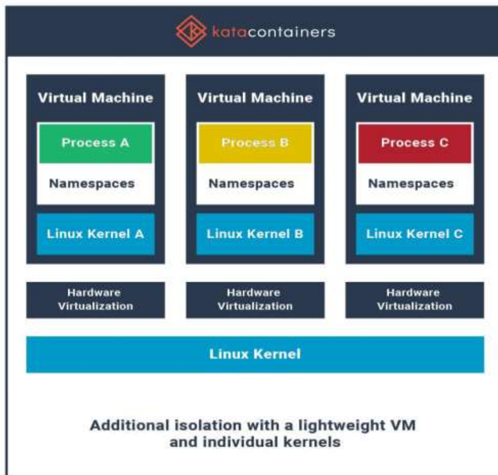
Figure 2.4: Containers running in isolated VM (Kata Containers, 2019c)
