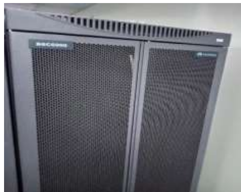
Plate I (b) BTS3900 (Closed Indoor BTS, Vendor: Huawei)
