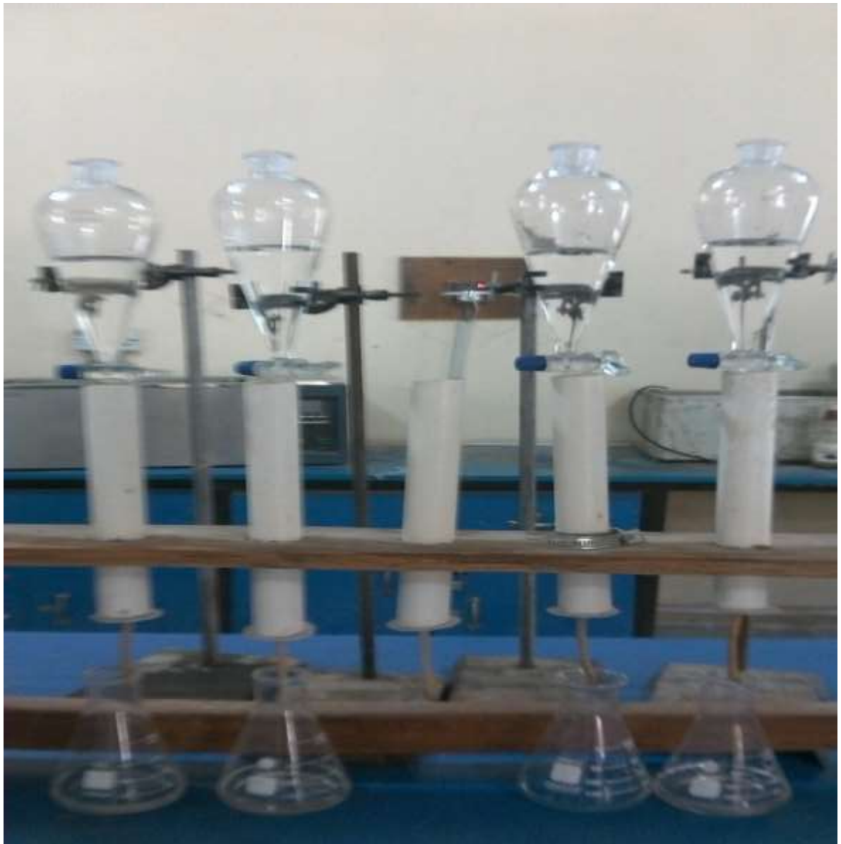
Plate I: Experimental setup for the percolating reactor column used in the study of the desorption rates of phosphates and nitrates from the soil and different fertilizer sources
