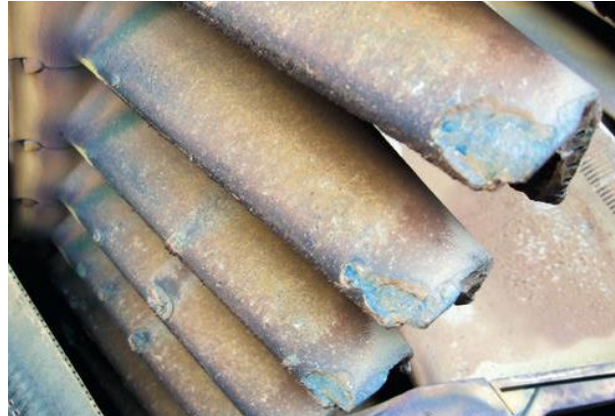
Plate 1: Degraded turbine blade tips (Bacos, 2011)
