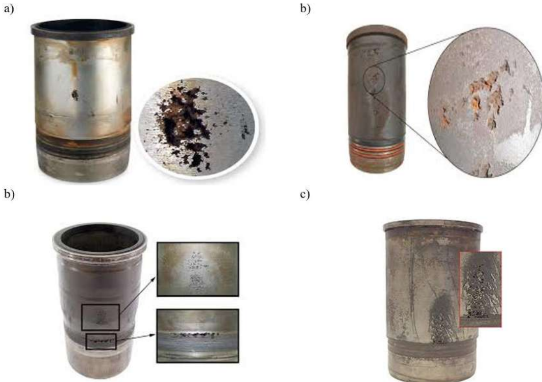
Fig. 2. Infected wet-cylinder liner
