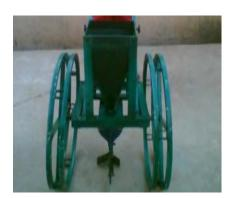
Plate II1: The Developed Manually Operated Single-Row Multi-Crop Planter
