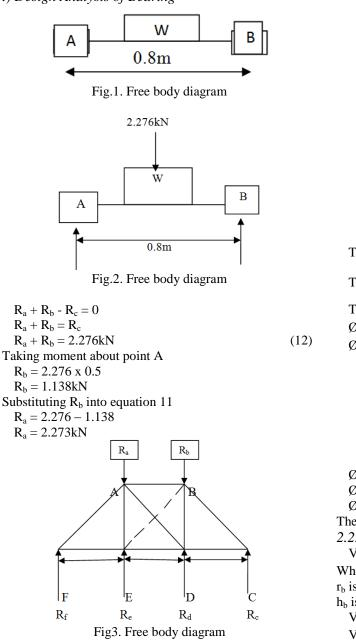
Since, upward forces is equal to downward forces  $R_{f} + R_{e} + R_{d} + R_{c} = R_{a} + R_{b}$ Where;  $R_{f} = R_{e} = R_{d} = R_{c} \text{ and also } R_{a} = R_{b} = 1.138 \text{kN}$ Then;  $4R_{f} = 2R_{a}$   $4R_{f} = 2R_{a}$   $4R_{f} = 2(1.138)$   $R_{f} = \frac{2.276}{4}$   $R_{f} = 0.569 \text{kN}$ Therefore,  $R_{f} = 0.569 \text{kN}$   $R_{b} = 1.138 \text{kN}$   $R_{c} = 0.569 \text{kN}$
