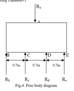
Downward forces is equal to the upward forces  $R_d + R_c + R_b + R_f = R_A \label{eq:result}$
