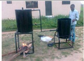
Fig 9: Equipment set-up for parboiling rice
