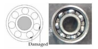
Figure 3: Diagram and plate of faulty [3].
