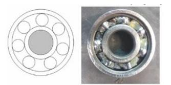
Figure 1: Diagram and plate of a healthy bearing [3].
