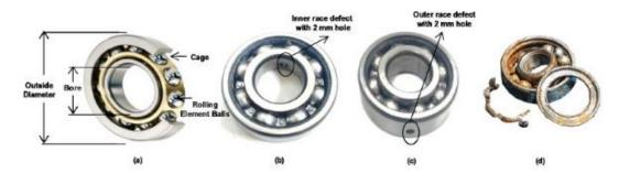
Figure 2: (a) Healthy bearing (b) inner race defect (c) outer race defect (d) lubrication defects [1, 8].
