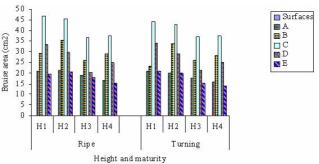
Figure 2. Effects of height, maturity and impact surfaces on the bruise area on the fruits
