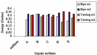
Figure 4. Effects of mass and impact surfaces on the energy absorbed by the fresh tomato fruits
