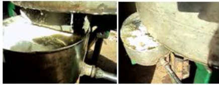
Plate II: Paste being expelled out of machine
